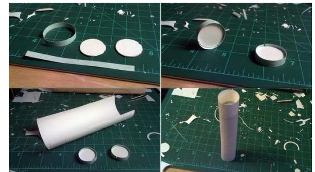
If the cylinder warps, wrap and glue a rectangle of mat board around it, but be sure to curl it tightly first. You can use rubber bands to secure it while it dries.
